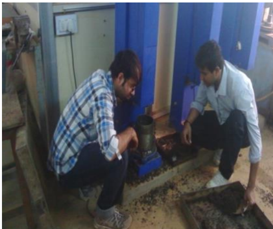
Photograph.1: Modified Compaction Test being Performed
